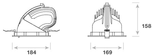
Abmessungen in mm / Dimensions in mm
