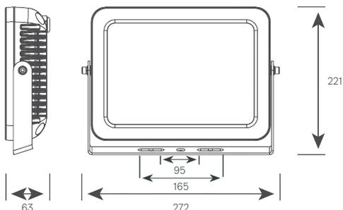
Abmessungen in mm / dimensions in mm
